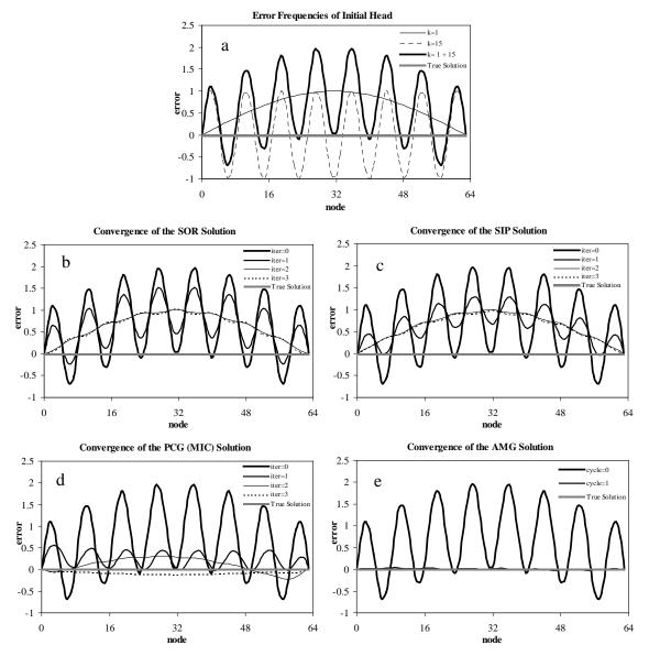
Figure 1. Errors in the solution to a one-dimensional flow problem with constant head boundaries of zero at both ends. (a) Components of initial head (errors), with smooth (k=1) and oscillatory (k=15) components. Reduction of error components for the (b) SOR, (c) SIP, (d) PCG2 with the modified incomplete Cholesky (MIC) preconditioner, and (e) AMG solvers.
